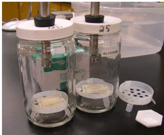
FIGURE 11: Examples of sample holders for powder, pellet, and liquid forms of VCI materials. (12)
