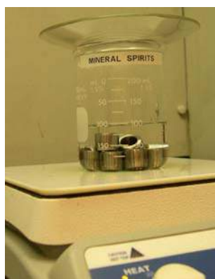
FIGURE 7: Hot plate with cleaning beaker covered with watch glass to reduce evaporation. (8)
