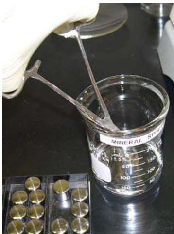
FIGURE 6: Forceps being used to place prepared steel specimens into the cleaning beaker. (7)
